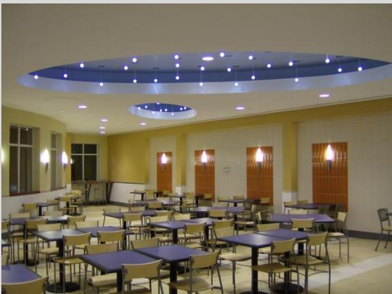
Taking an older design and introducing new technology is a natural direction for Terry. For Cumberland Mall, the original design had incandescent lamps on stems. In keeping with the architectural (TVS&A) intent, Terry created LED modules with an acrylic sphere at each end. The concept was eventually turned into a standard product offering by the manufacturer.
